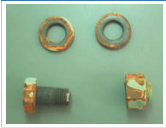
Figure 3-30: Sample bolt with delayed fatigue fracture
