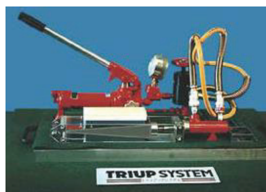
Photo 3-16: 50 Ton Hydraulic Jack
